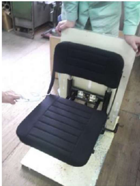
To fix swivel parts (5/8"-11 UNC)
