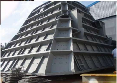
Hopper liner HLN M16 SS400/HDZ
