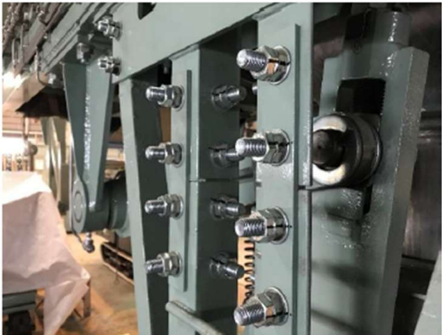
Coal Charging Car HLN M8~M33 SS400, SUS304
